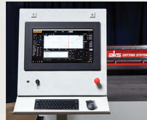
19" Industrial Touchscreen Operator Console with the FlashCut Pro CNC integrated all-in-one CAD/CAM/CNC software.
