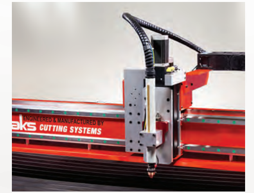
Z-axis carriage automatic lifter with torch height control (THC), magnetic breakaway head, laser pointer and plasma torch
