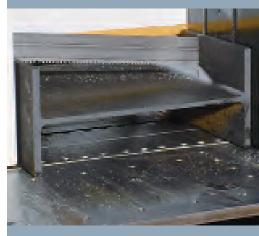
The saw head swings up to 60° both ways with programmable go-to settings for versatile production cutting while reducing material handling time.
