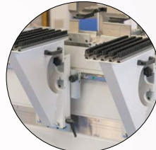
Front Support Arms (With Brushes and Height Adjustment)
