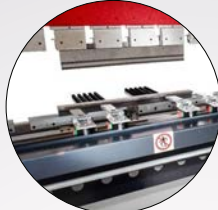
2 Axis Back Gauge (4 fingers) X, R
