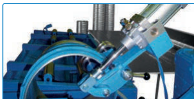
Automatic Corrugation Unit Produce ducts with smooth inside surface at the ends but reinforced with corrugation
