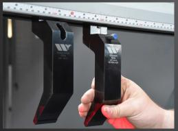
TOOL USAGE FLEXIBILITY – Machines equipped with the ATC are not limited to using tools from the tool changer's storage. The operator can use the machine as a stand-alone press brake, as well as an automated system. This give the operator flexibility for hot jobs, one-offs, or jobs that utilize tooling not stored in the tool changer.
