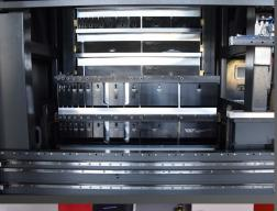
AUTOMATED TOOL SETUP/CLEANING — The Tool Changer will automatically change tooling, while the operator is free to perform other tasks, further reducing press brake setup time. Up to 50mm (2") V-die opening and 500mm (19.7") tooling lengths can be picked and placed due to the single, large capacity tool manipulator. The manipulator is also equipped with a die bed cleaner that runs automatically during tool changes.
