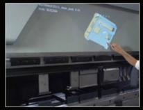
The two-dimensional sensor makes the ram a big touch screen
