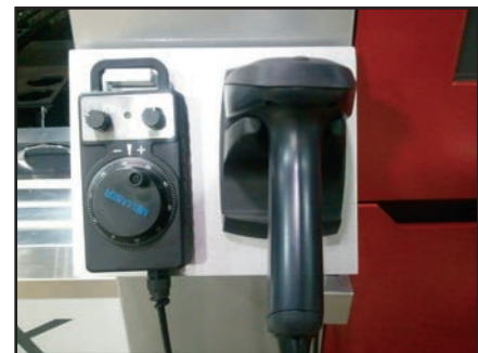
Handle Box and Bar Code Reader combine for a more user friendly experience.
