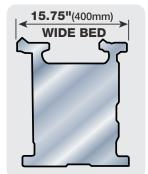
Extra heavy-duty 15.7" (400mm) wide bed gives our machines the capability of withstanding heavy use and excellent durability with minimum maintenance over many years.
