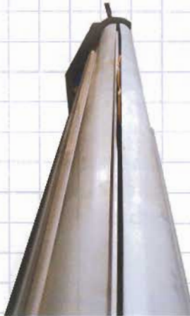
Notice straight seam as part nears completion.
