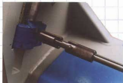
Bending Roll Drive disconnect collar with detent position to allow tilting the back roll for rolling cones and similar parts. (Shown disconnected for tilting.)
