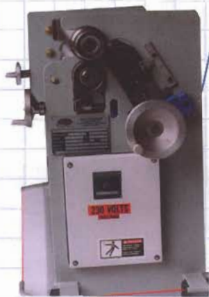
Drop end view of B machine shows location of electrical box, pinch roll adjusting hand wheel, and position scale. Notice the alloy steel bearing case and wedge screw arrangement for accurate positioning of the pinch roll.
