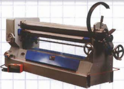
B-6-72 (7/32 x 6') with extended shafts, and bar and angle attachment.
