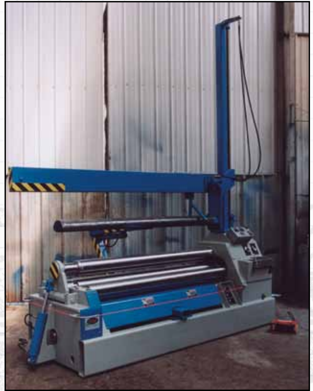
403-6-8 (.140" x 8') with 1 side support, 1 overhead support, ejector, 421 digital readout with foot pedal. This machine is used to manufacture produce harvesting equipment.
