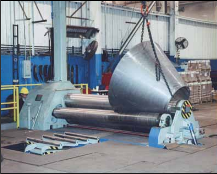
403-16-10 (57/64" 10') with side and overhead supports used to manufacture silos and related parts for asphalt production.
