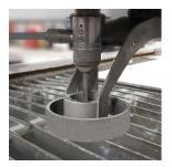
**Automatic Touch Probe and Collision Sensor Bracket** – automatic step touch probe can be programmed at certain distance intervals to engage and insure proper nozzle tip stand-off height control and then adjusted while cutting to compensate if the work piece material is warped or not flat. The collision sensor ring can detect most crashes of the nozzle into tipped-up parts, or other items, via a circular metal ring around the nozzle tip which is pneumatically engaged and easily reset.
