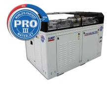
**Upgrade to 90,000 psi** – waterjet cutting with ultra-high pressures of 90,000 psi offers users the latest technology to maximize cutting speeds. For example, 90,000 psi cutting of 1" aluminum is 15-25ipm while 60,000 psi cutting of 1" aluminum is 5 -10 ipm. With the latest technology from KMT in high pressure seals, cylinders and check valves, operating costs of the 90,000 psi operation have never been lower, and usually cost only a few dollars more per hour than a 60,000 psi operation.
