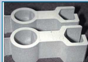
3/4" stainless steel cut with 60K with smoothest edge
