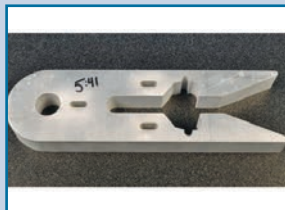
1" aluminum with 1/2" slots and 1 inch hole cut with 90K
